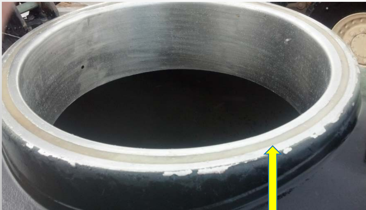
Gasket level without excess sealant
